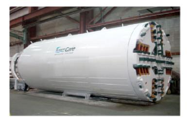
Figure 1 EPB Tunnel Boring Machine ready for use on Project Hobson
